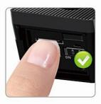
Please Insert the TF card in the correct direction and use the tip of your fingernail to push it into the slot, if the TF card can fit in the slot, means installation successfully. To remove TF card, use your fingernail to push it inward to eject and take it out.
